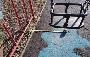
**Finding:** The surfacing width under each seat is less than 1.75 metres and fails the requirements of BS EN 1176 Part 2
